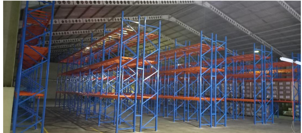
Selective pallet rackLoad 2000kg/level
